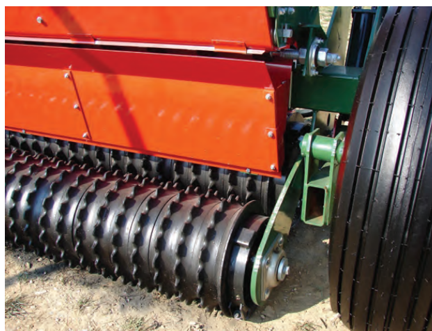
Figure 6.4. Double-corrugated roller-seeder (Brillion brand).
